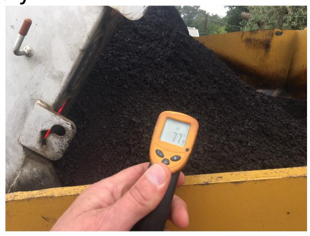
Heat sensing showing 76.8 F during the paving process.
